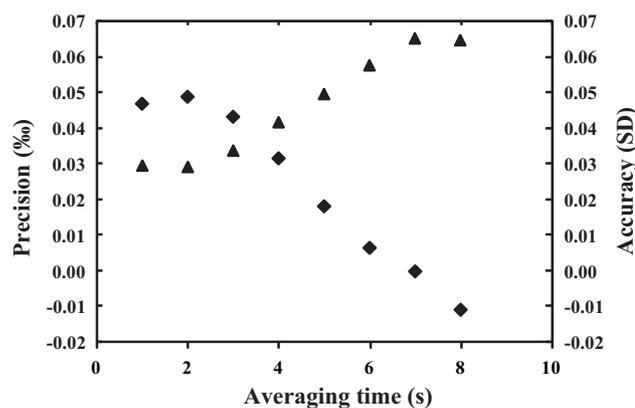
**Figure 3.** Accuracy (diamonds) and precision (triangles) of  $\delta^{13}\text{C}$  measured from pulses of standard gases ( $n = 12$ ) as a function of averaging time. For 'accuracy',  $\delta^{13}\text{C}$  was averaged over 1 to 8 s and compared with the known value of the standard gas. 'Precision' is the standard deviation of the respective period (10 Hz sampling rate).
