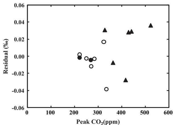
**Figure 2.** Difference between measured and known  $\delta^{13}\text{C}$  values for pulses of known standard gases (filled circles: 350 ppm,  $-11.21\text{‰}$ ; open circles: 550 ppm,  $-11.12\text{‰}$ ; triangles: 750 ppm,  $-11.07\text{‰}$ ). Peak CO<sub>2</sub> concentrations are lower than standard concentrations due to dilution with CO<sub>2</sub>-free medical air that was used as carrier gas.
